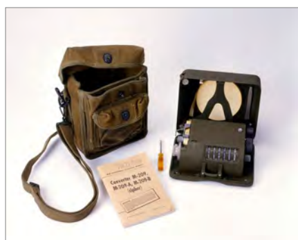
M-209 Cipher Machine (c. 1943, US Army)
